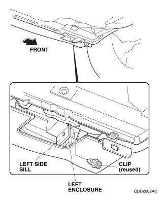
19. Secure the front of the left side sill with the one clip and two self-tapping screws removed in step 1.
